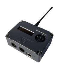
The ODU is a 1W UHF transmitter which benefits from a wide RF bandwidth of 403-473MHz giving superior frequency flexibility. It is powered by either 12v 4 pin XLR or PoE and the data connection from the IDU can be either RS232/485 or Ethernet. Multizone is a feature whereby multiple ODUs operate on different frequencies in different zones. This enables coverage of very wide areas such as golf courses.
