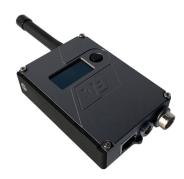
The RX-SM is the camera mounted data receiver. It can be supplied as a stand alone unit or integrated into the OBTX, Sapphire BTX or Eclipse TX transmitters. In multizone mode the receiver is programmed with multiple frequencies and it switches at a predefined SNR level.
