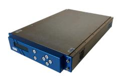
The IDU can be connected to OCPs via legacy RS data or Ethernet and it works with the manufacturers own OCP. Up to 4 cameras on a single RF channel can be controlled and bothRed & Green tally are supported.
